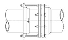
6) Install the remaining MJ bolts and evenly tighten all follower gland nuts to AWWA standards for mechanical joints.
