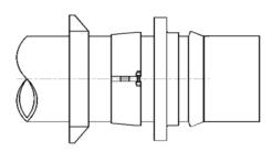
1) Install, in order, onto pipe spigot: casing gland, inner serrated ring, mechanical joint follower gland and gasket.
